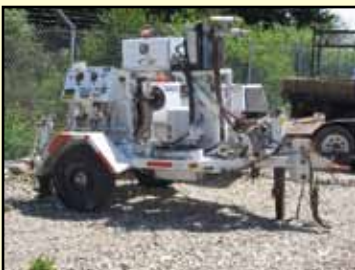
1998 TSE Cable Puller
